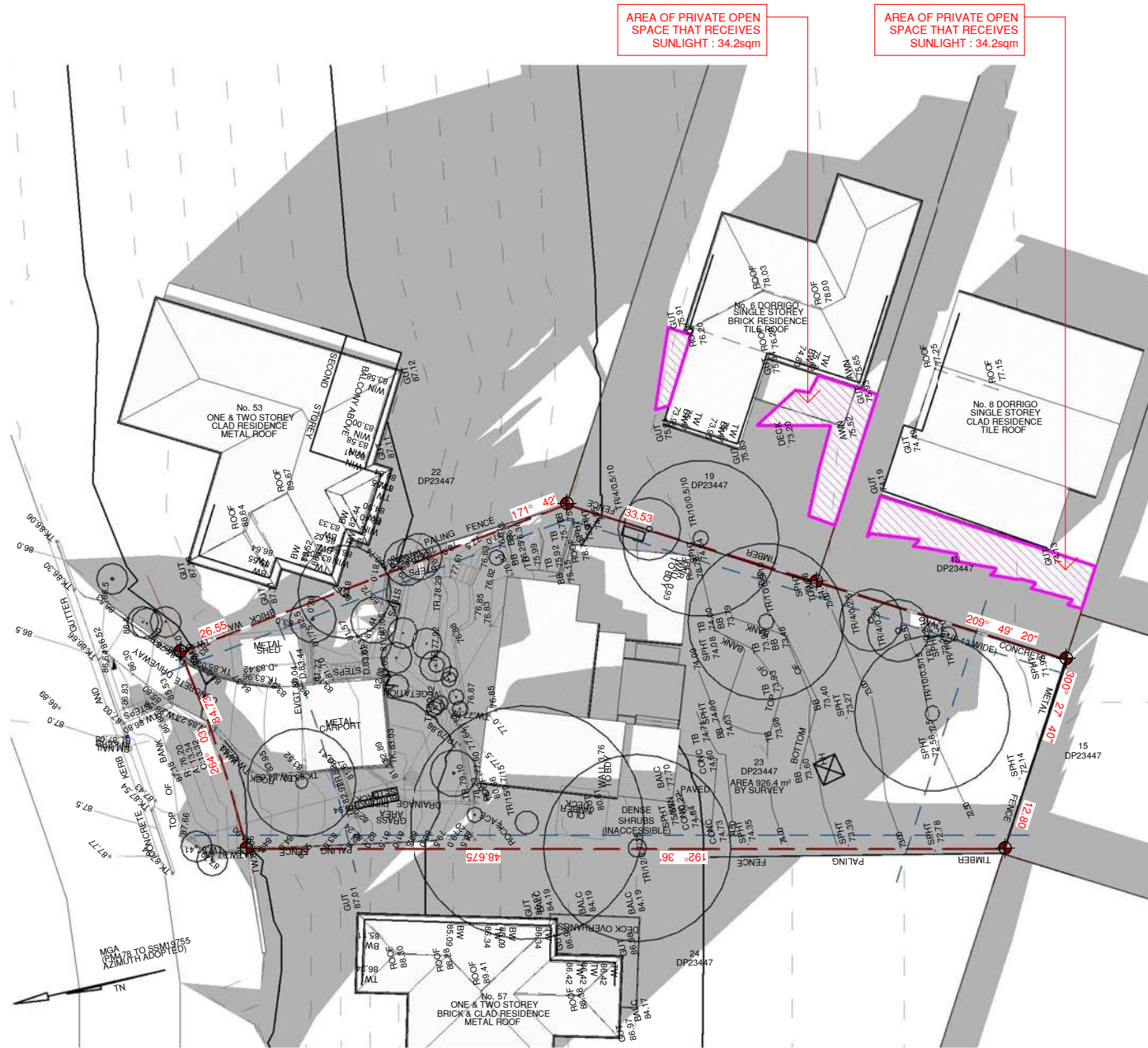
1 SHADOW DIAGRAM 21 JUNE - 2PM - EXISTING 1 : 400
