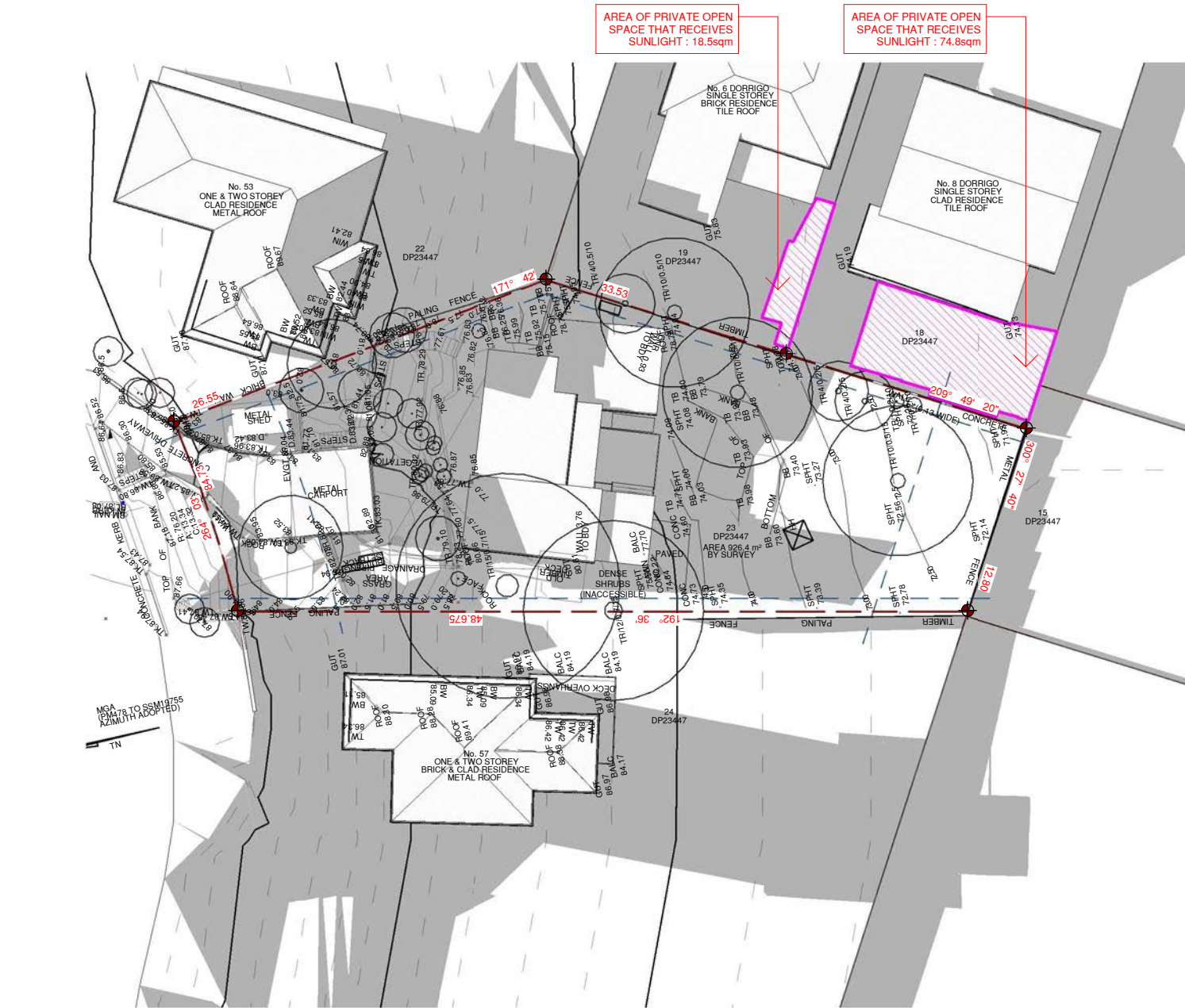
1 SHADOW DIAGRAM 21 JUNE - 10.30AM - EXISTING 1 : 400
