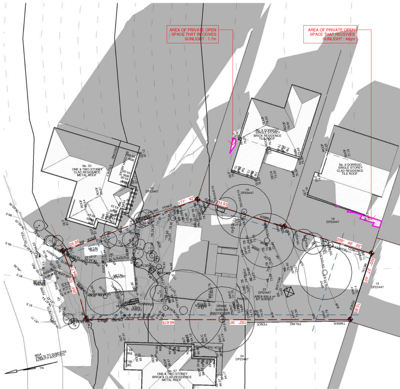
1 SHADOW DIAGRAM 21 JUNE - 3PM - EXISTING 1 : 400
